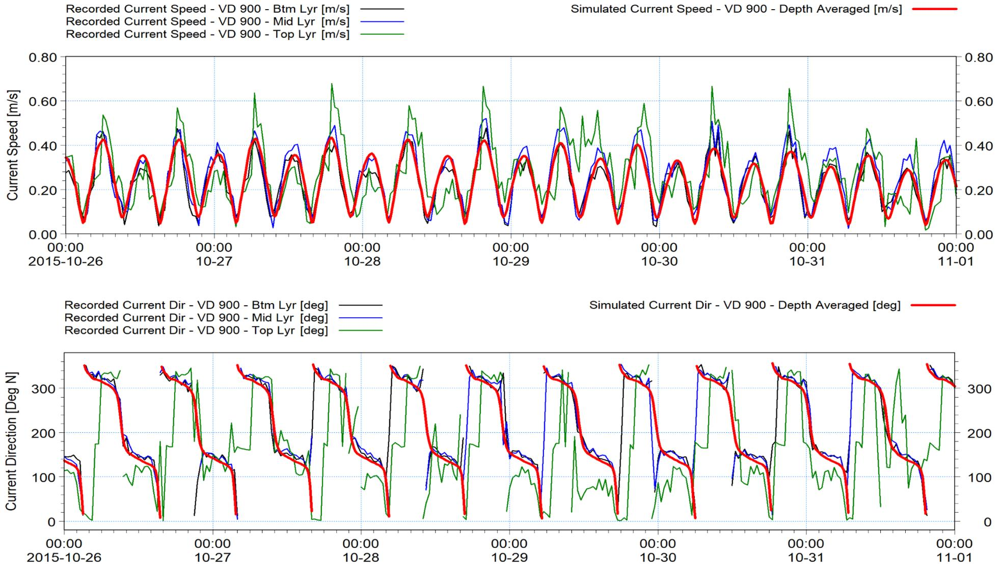
Figure 8: Comparison of recorded and simulated current speeds (upper) and directions (lower) at VD 900 -Spring Tides
