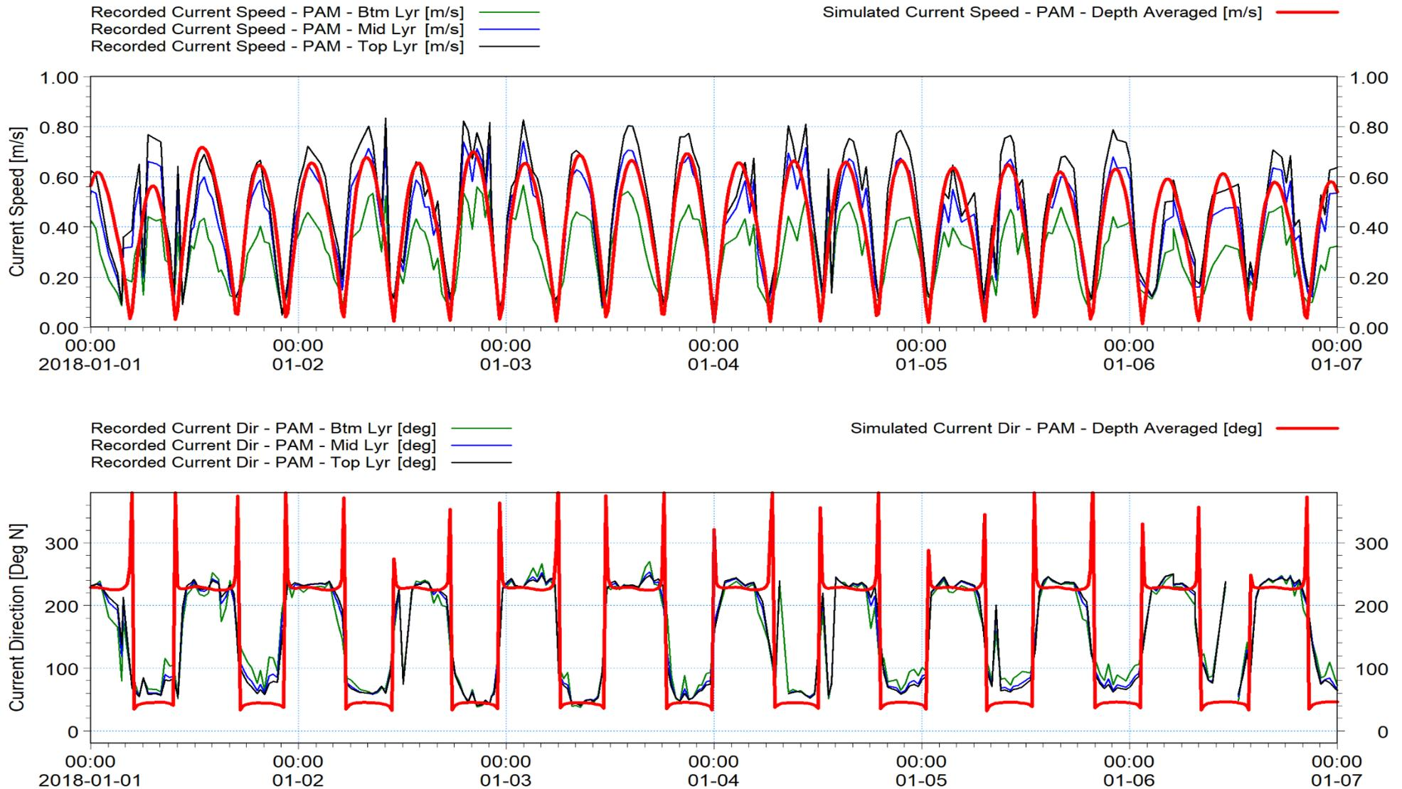
Figure 9: Comparison of recorded and simulated current speeds (upper) and directions (lower) at PAM Site -Spring Tides
