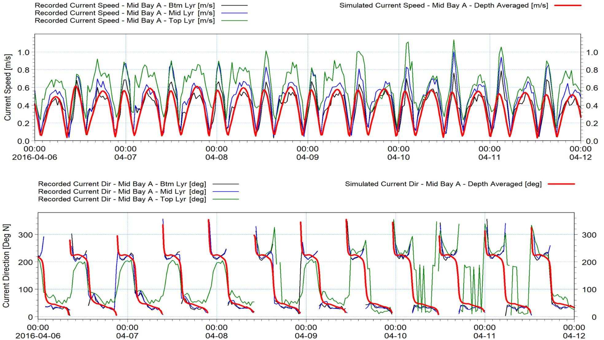
Figure 6: Comparison of recorded and simulated current speeds (upper) and directions (lower) at Mid Bay A - Spring Tides
