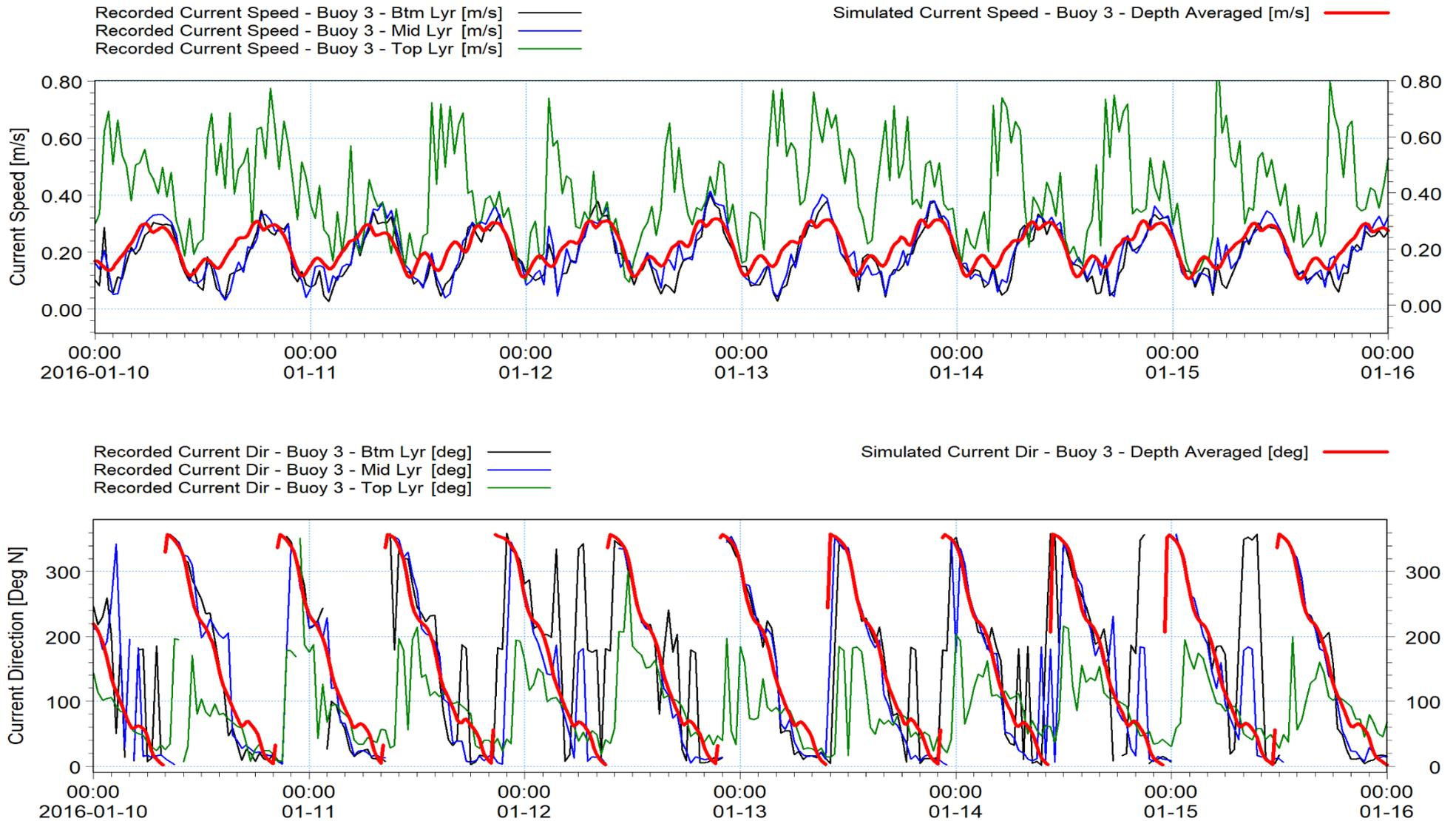
Figure 4: Comparison of recorded and simulated current speeds (upper) and directions (lower) at Buoy 3 - Spring Tides
