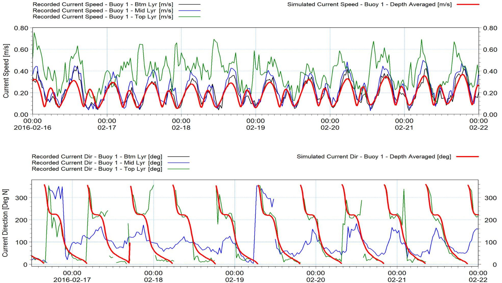
Figure 10: Comparison of recorded and simulated current speeds (upper) and directions (lower) at Buoy 1 -Neap Tides
