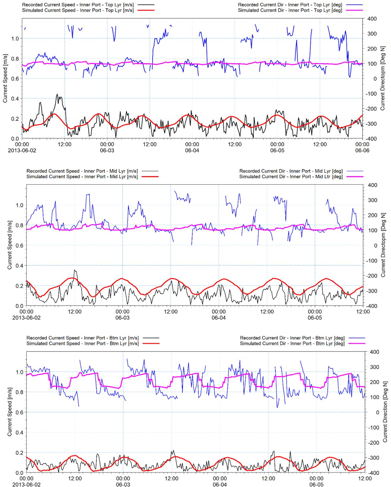
Figure 18: Comparison of recorded and simulated current speeds and directions throughout the top, middle and bottom layers of the water column at the Inner Port ADCP - Neap Tides
