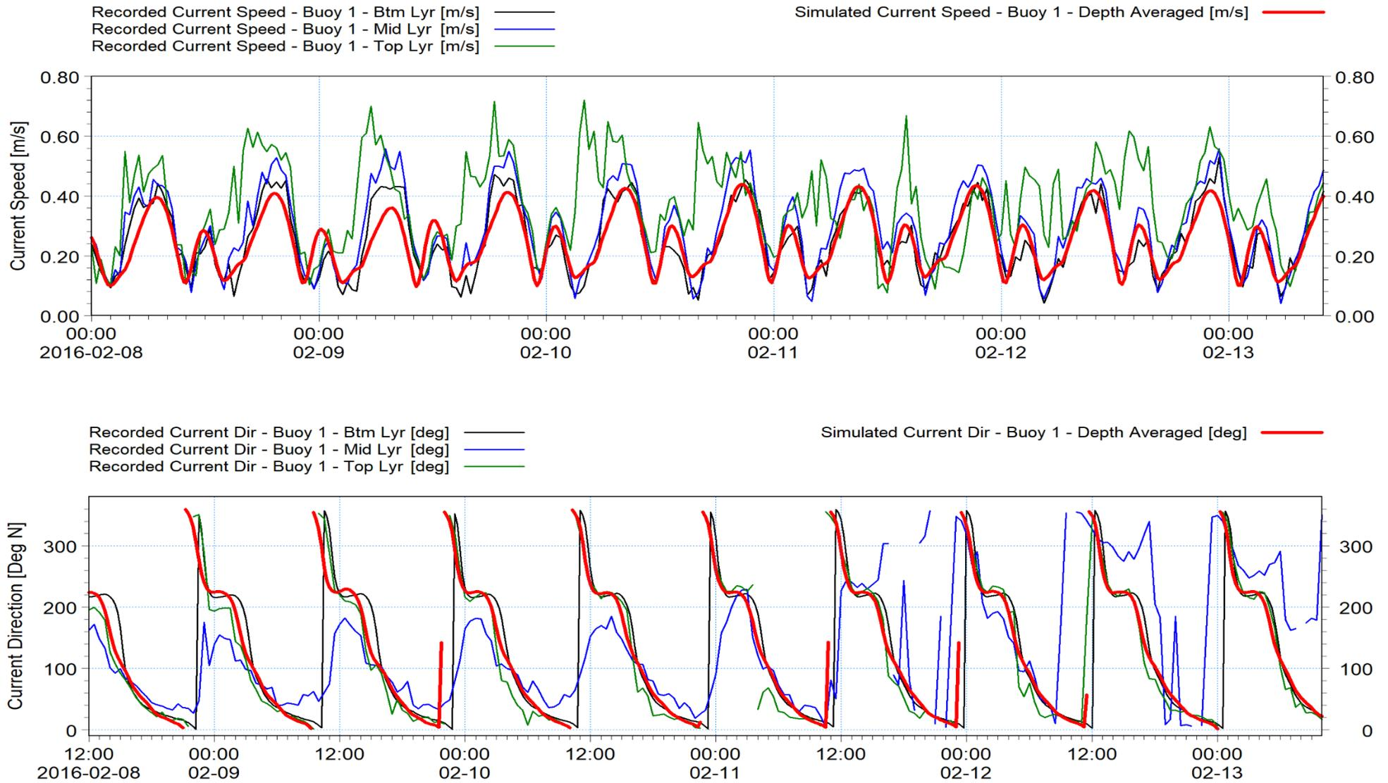
Figure 3: Comparison of recorded and simulated current speeds (upper) and directions (lower) at Buoy 1 - Spring Tides
