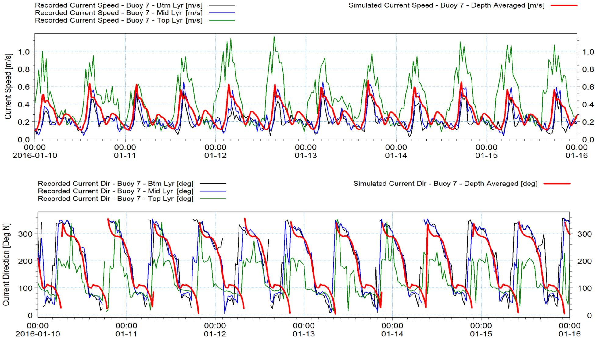
Figure 5: Comparison of recorded and simulated current speeds (upper) and directions (lower) at Buoy 7 -Spring Tides
