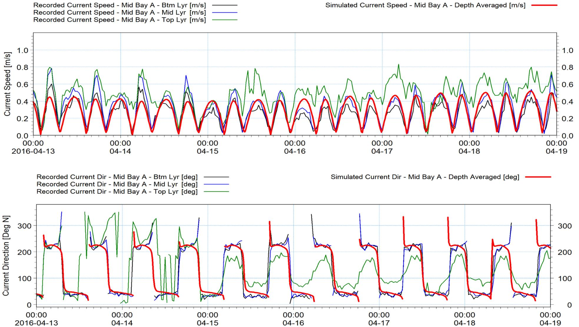
Figure 13: Comparison of recorded and simulated current speeds (upper) and directions (lower) at Mid Bay A -Neap Tides
