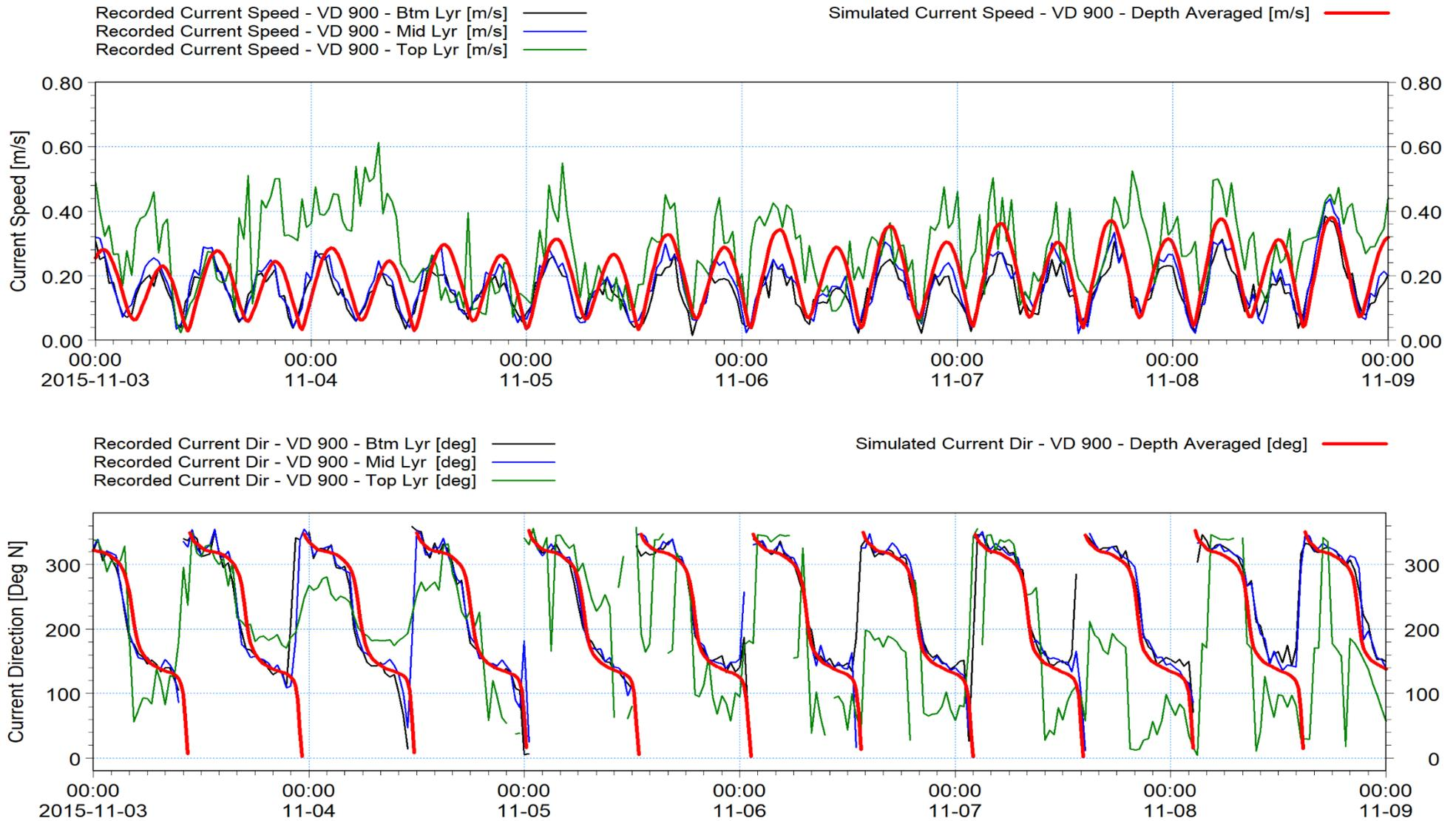
Figure 15: Comparison of recorded and simulated current speeds (upper) and directions (lower) at VD 900 -Neap Tides
